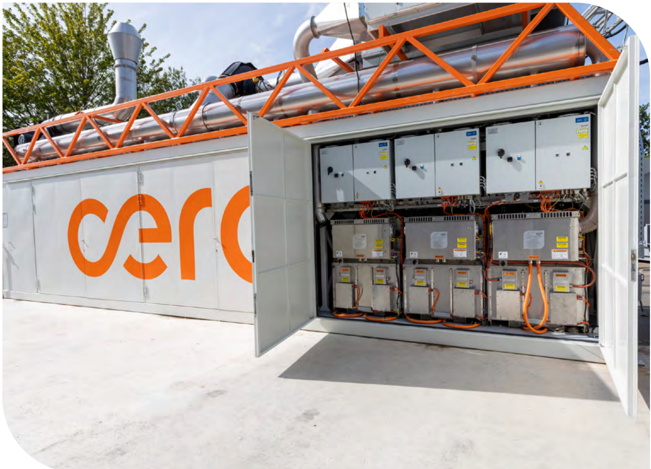
Figure 14: 1 MW Ceres SOEC system demonstrator operating at Shell's R&D site in Bangalore, India. Image courtesy of Shell Plc.
